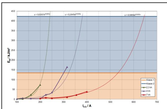
Fig. 10: Incident energy to be expected in dependency on NH fuse rating (measured values and extrapolation functions for the different short-circuit currents), gG fuses
