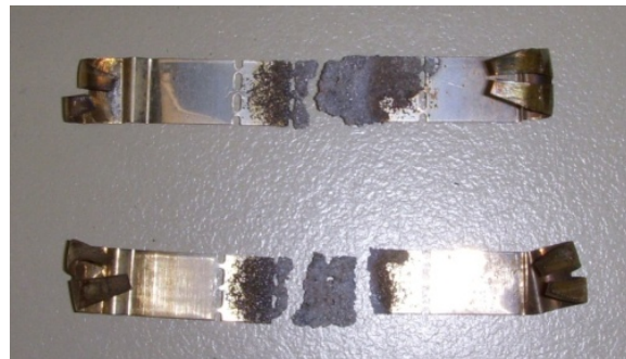
Fig. 9: Melting element after incorrect overload operation
