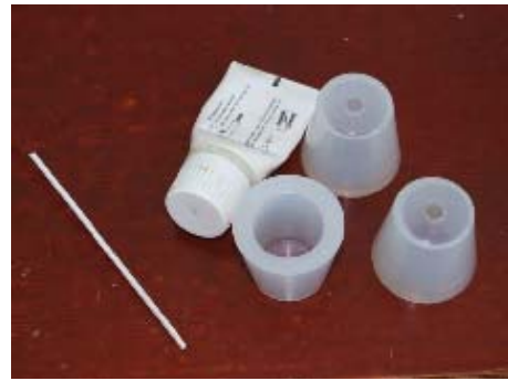
Figure 10: Silicon insertion, silicon lubricant and tube for silicon venting at installation onto the transformer's bushing
